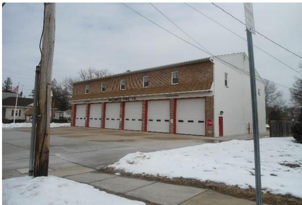
The roof's runoff could be stored in a rainwater harvesting system to be used for washing trucks. A bioretention system could be installed to manage runoff from the northern lot. The eastern portion of the lot could be replaced with grass pavers. A preliminary soil assessment for this site suggests that the site's existing soils have suitable drainage characteristics for green infrastructure.
